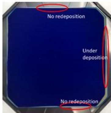
Large wafers tend to bend leading to significant underdeposition
