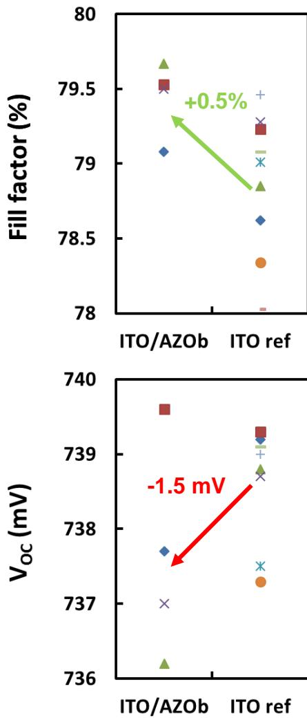
Replacement of ITO back contact via AZO leads to an efficiency gain of 0.45%
